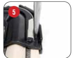
To open the part insert a flat screwdriver as shown and gently twist the tabs away from the part. Prying two tabs on the same side is generally all that is needed to remove the top.
