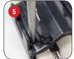
To open the part insert a flat screwdriver as shown and gently twist the tabs away from the part. Prying two tabs on the same side is generally all that is needed to remove the top.
